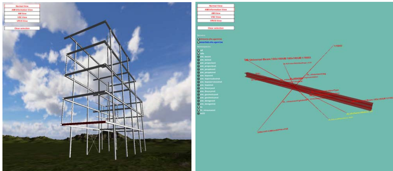
Fig. 2 Virtual world with the building structure of the visualized design, both in an overall First Person View (left) and in an isolated view for the building element highlighted earlier in Fig. 1 (right).
