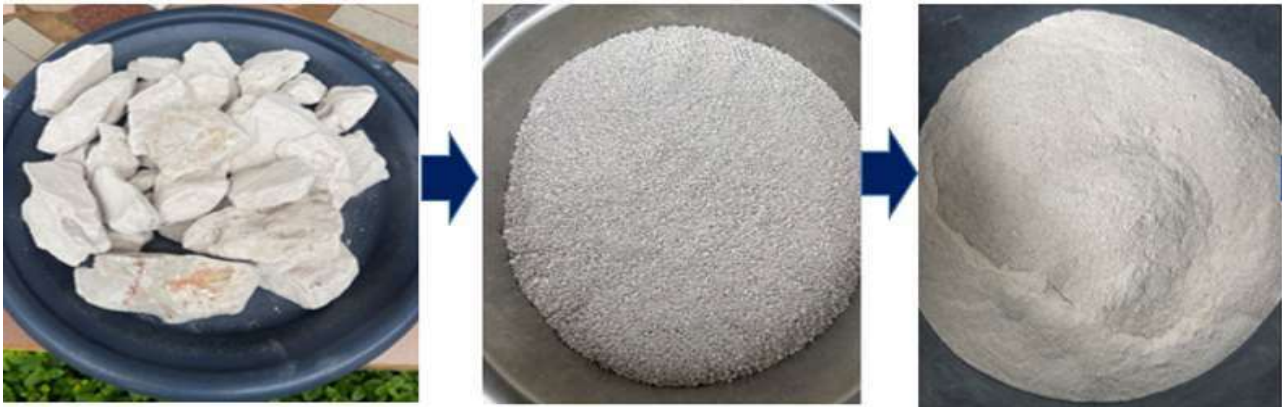
Fig. 2 Grinding of kaolinite clay.
