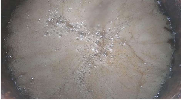
Fig. 4 Melted LDPE packaging.
