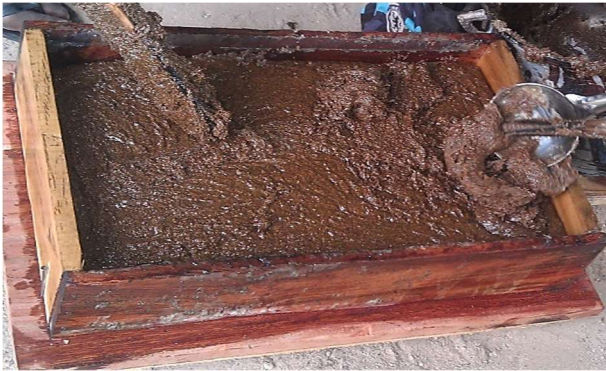
Fig. 5 Wood sawdust-plastic mix during molding.
