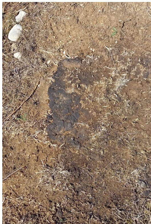
Fig. 10 Asphaltenes in the upper part of the soil.
