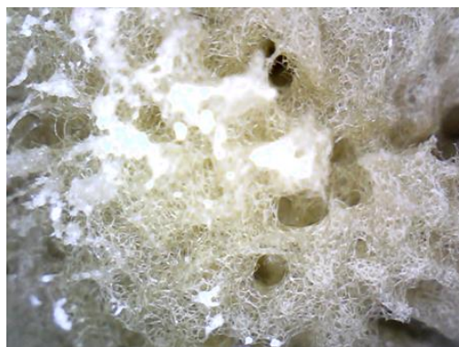
Fig. 11 Calcareous deposit after S1 spraying on the sponge spike.
