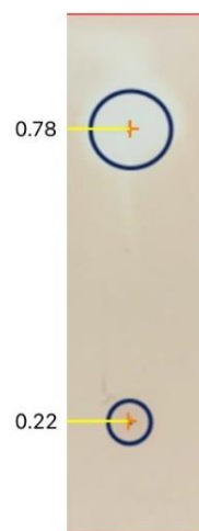
Fig. 6 TLC test to separate S1 and S2 protein fractions.
