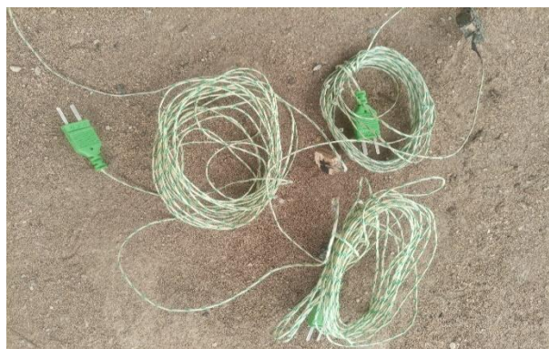
Fig. 7 K type thermocouples used for the temperature measurements.
