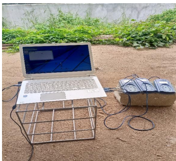
Fig. 8 Temperature data recording using a data logger USB-TC08 connected to a computer.
