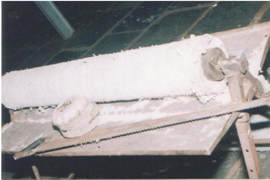
Fig. 7 Finished roller is ready for grooving operation using a band saw for grooving chrome composite leather cladding rollers commonly used in Indian roller ginning factories.
