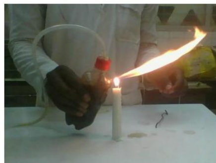
Fig. 4 Flammability test of biomethane.
