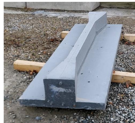
Fig. 5 Testing specimen made of UHPFRC before casting the over-lays.
