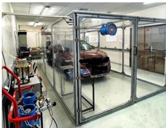
Fig. 1 Final assembly of the measurement platform (the Estaca's bubble).
