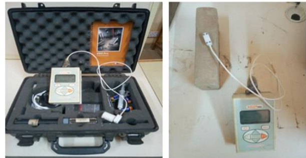
Fig. 3 Measurement of thermal properties with KD2-Pro.
