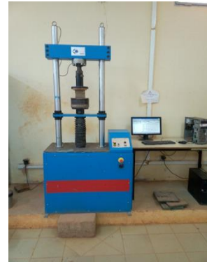
Fig. 2 Automatic hydraulic press with 3,000 kN of capacity.
