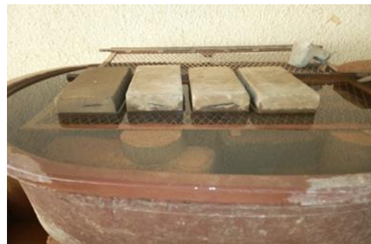
Fig. 4 Device for the test of water absorption by capillarity.
