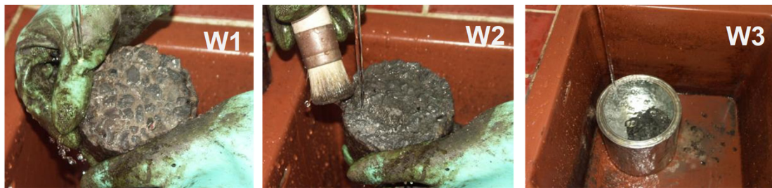
Fig. 2 Three methods of cleaning specimens after exposure.
