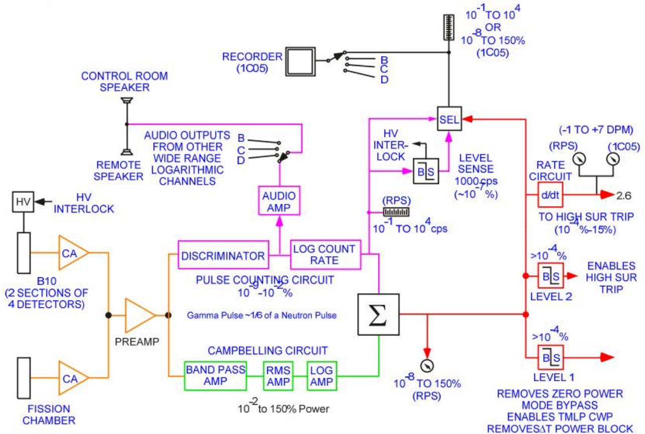
Fig. 11 Excure NI wide range logarithmic channel block diagram.
