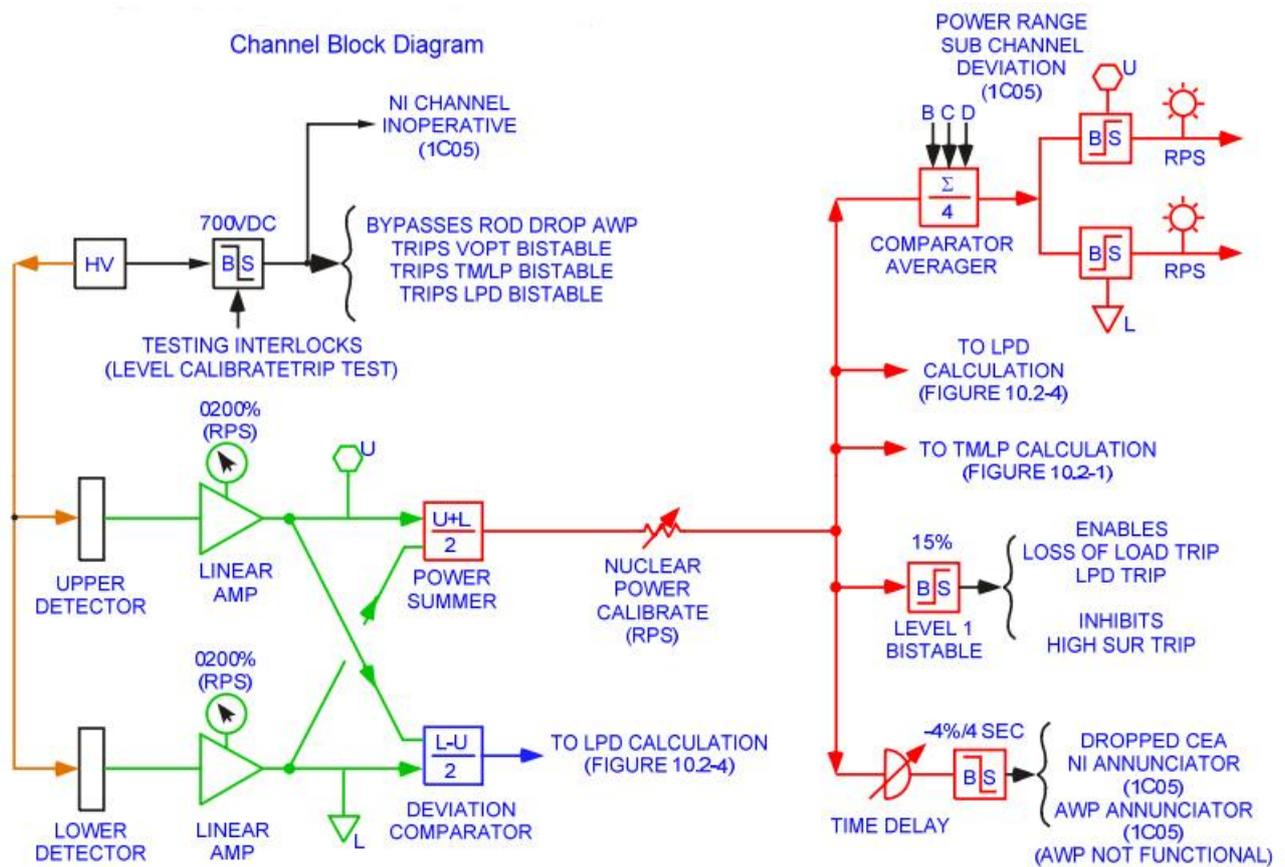
**Fig. 19 Excore nuclear instrumentation narrow range linear.**
