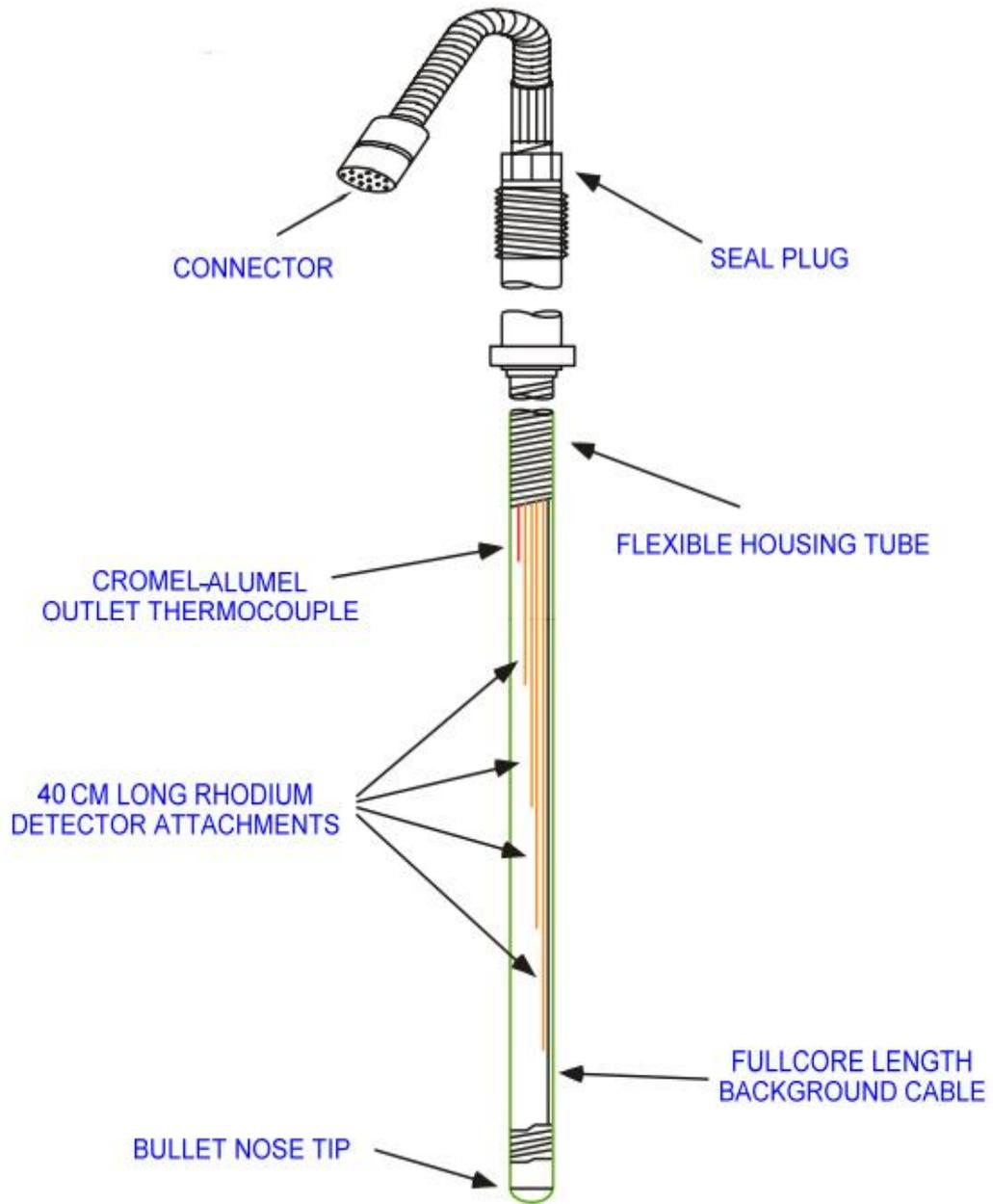
Fig. 25 Incore detector assembly.
