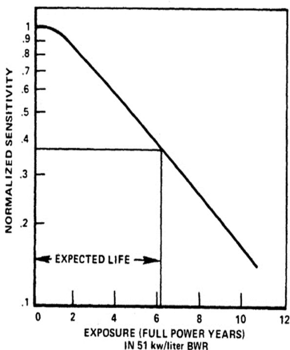
Fig. 2 Wide range sensor burnup characteristics.
