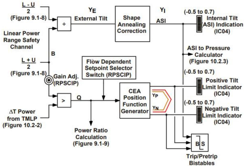
Fig. 15 Local power density trip diagram.
