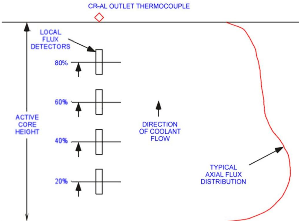
Fig. 24 Incore detector axial arrangement.
