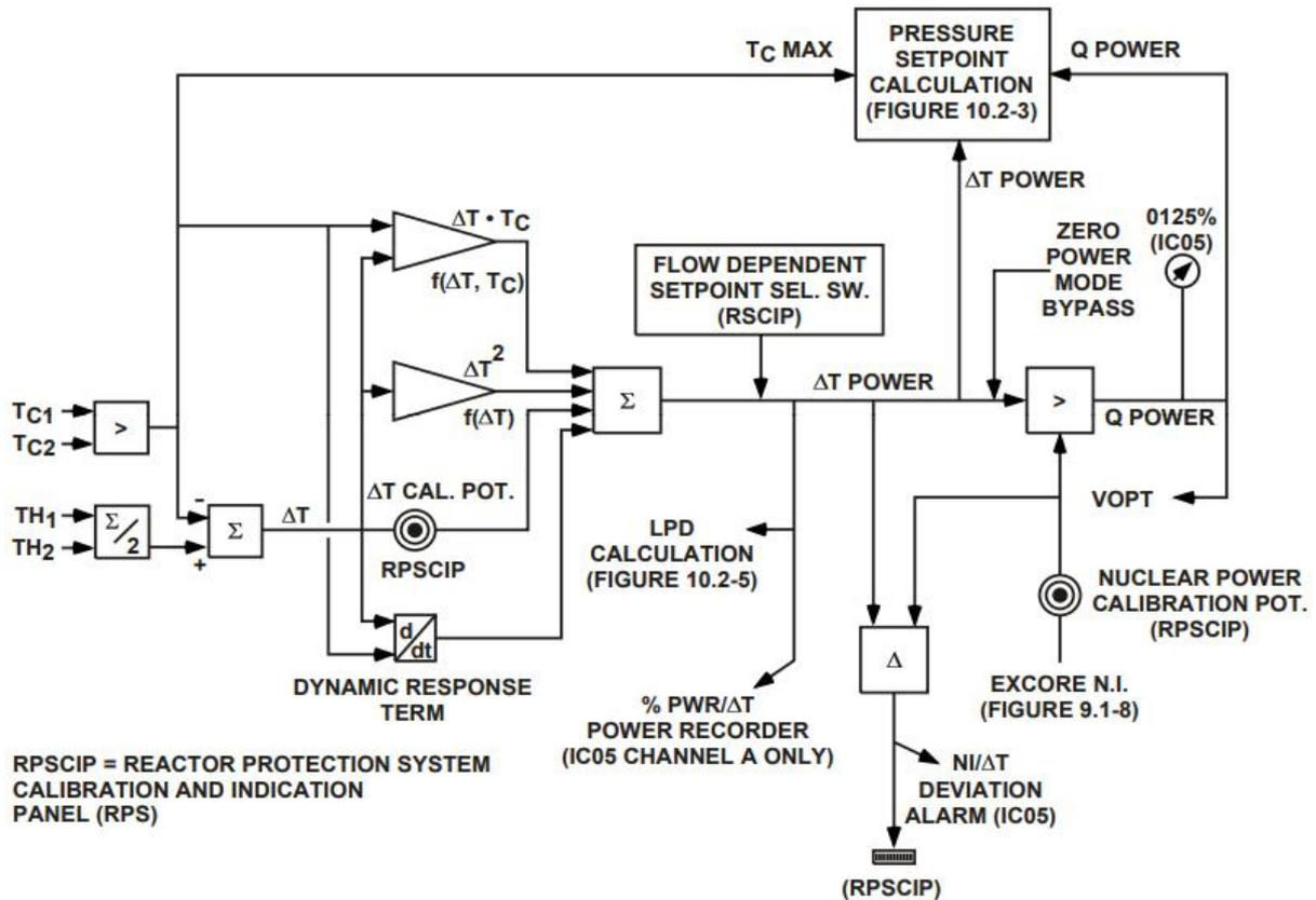
Fig. 13 TMLP ΔT power calculation diagram.
