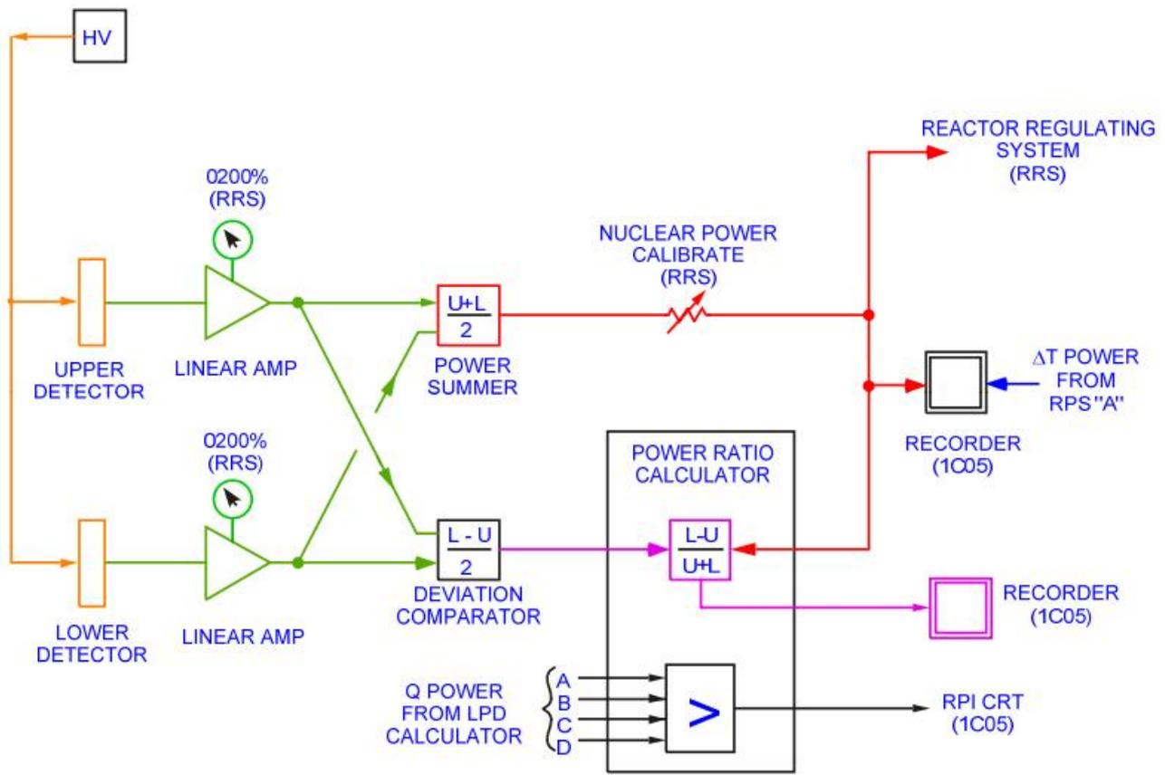
Fig. 20 Linear power control channel block diagram.
