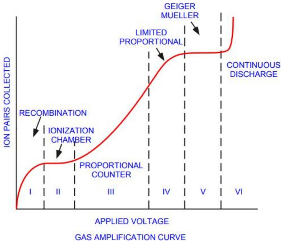
Fig. 7 Ion pairs versus applied voltage.
