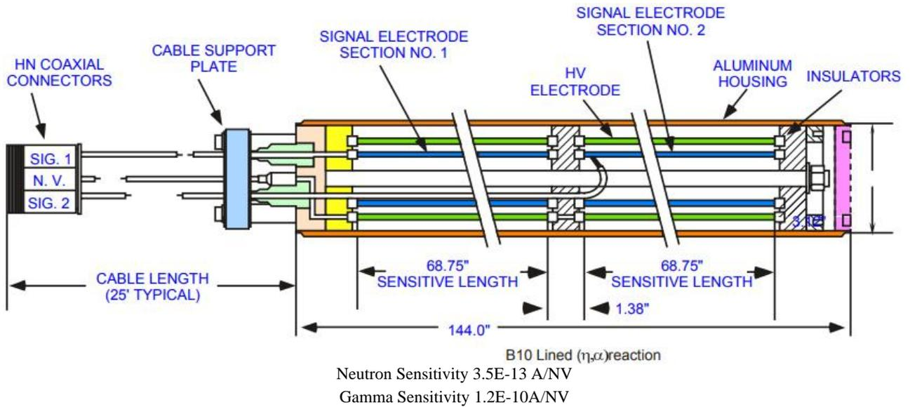
**Fig. 18 Uncompensated ionization chamber.**
