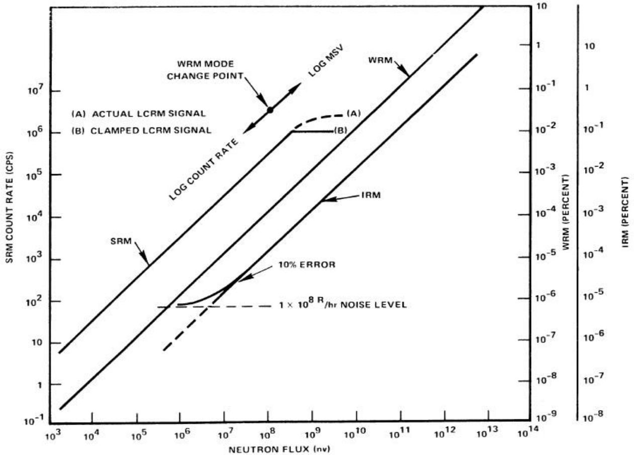
Fig. 5 Linearity of WRNM channel.
