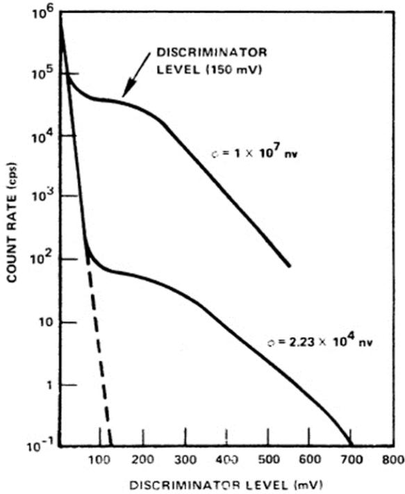
Fig. 3 Integral pulse height distribution Aerotest factor.
