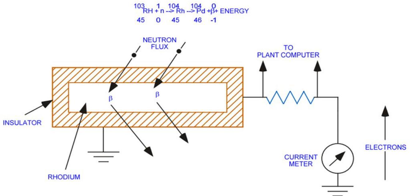
Fig. 21 Self-powered neutron detector.
