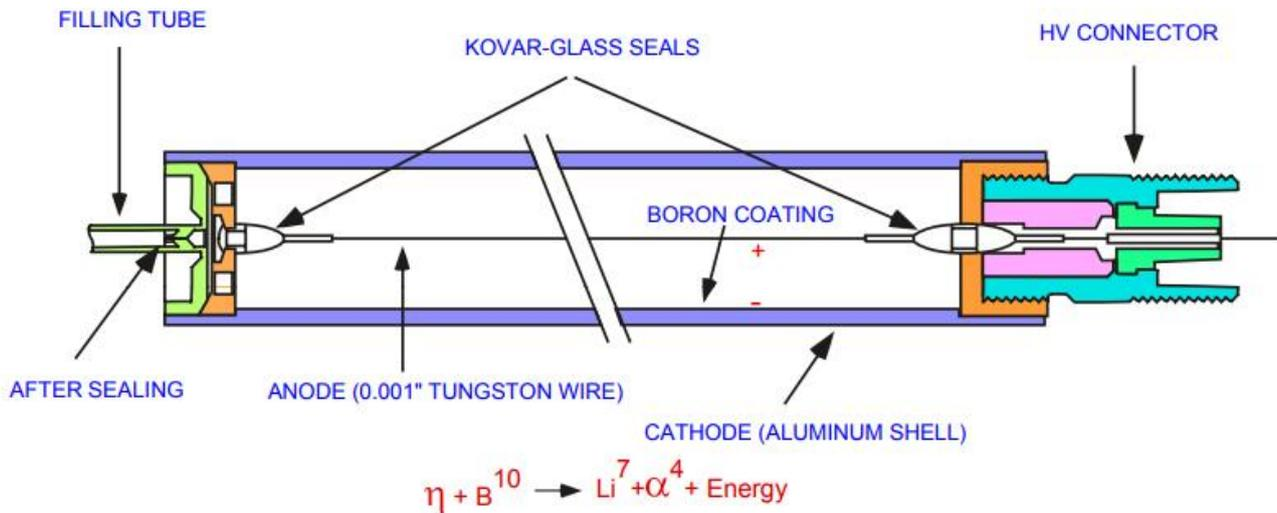
Fig. 9 Typical B10 proportional counter nuclear instrumentation.
