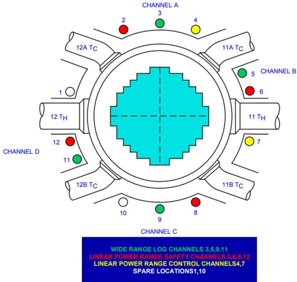
Fig. 8 Excore detector location.
