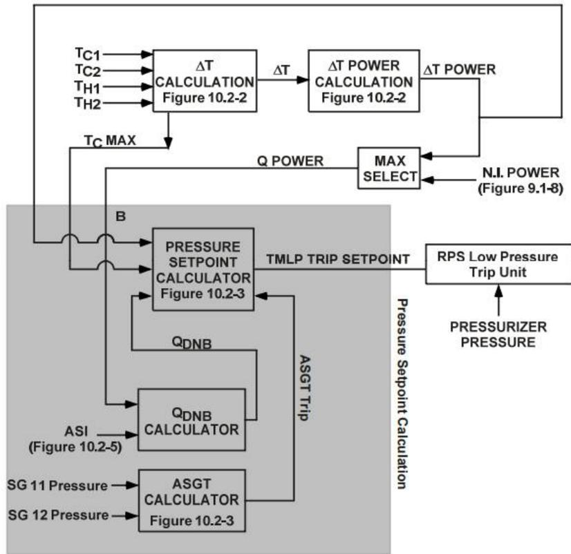
Fig. 12 ΔT/TMLP calculation block diagram.
