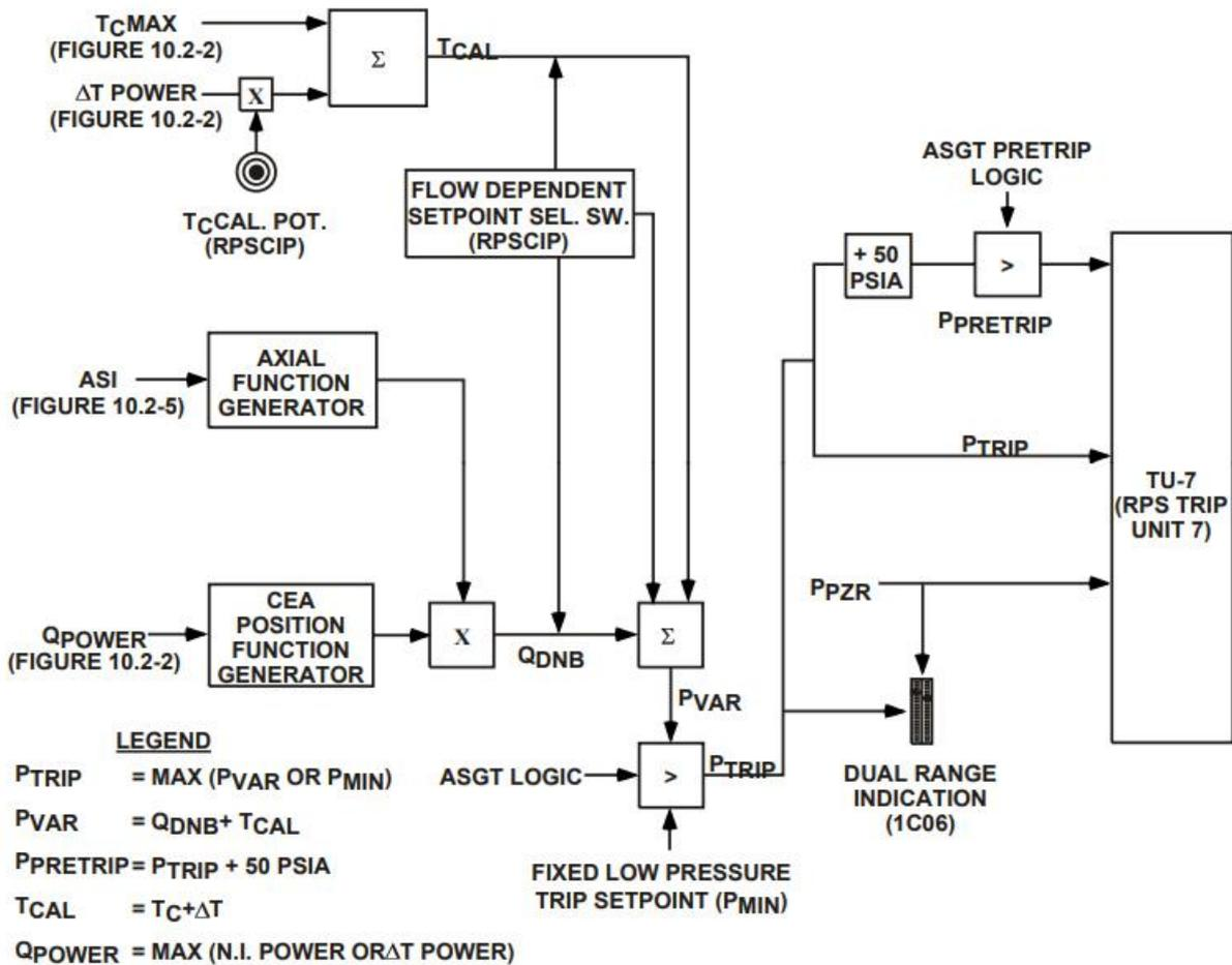
Fig. 16 TMLP pressure setpoint calculation.
