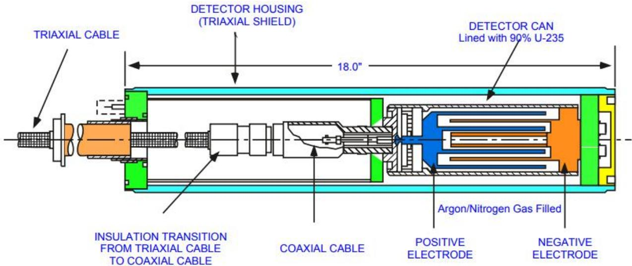
Fig. 10 Fission chamber (neutron sensitivity 0.7 Counts/nV) schematic.
