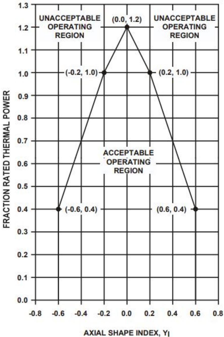
Fig. 14 Axial shape index boundary diagram.
