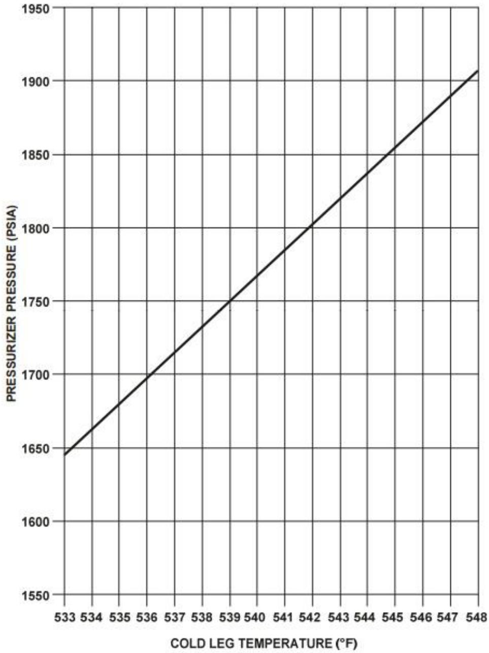
Fig. 17 Pressure setpoint versus temperature.
