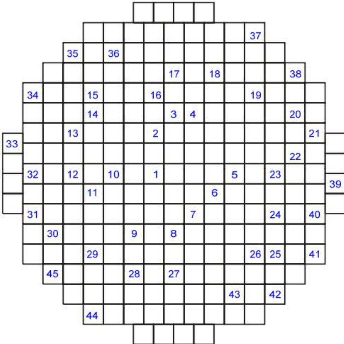
Fig. 26 Incore detector location.
