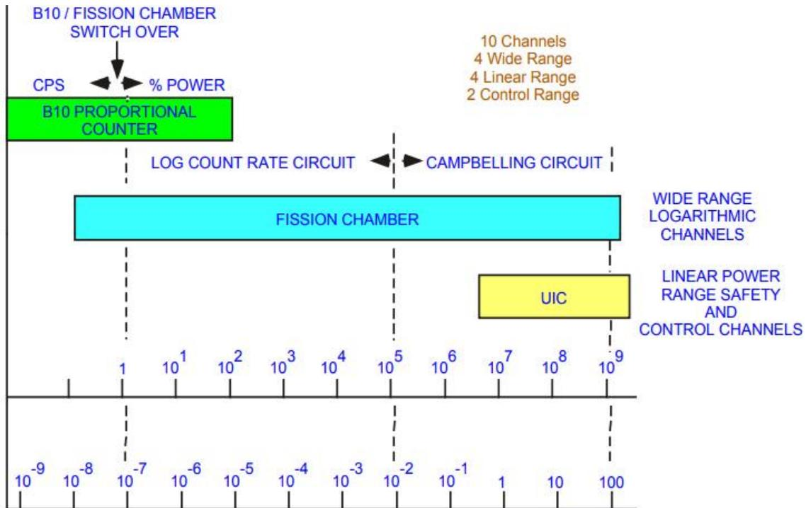
**Fig. 6 Typical flux coverage with detectors.**
