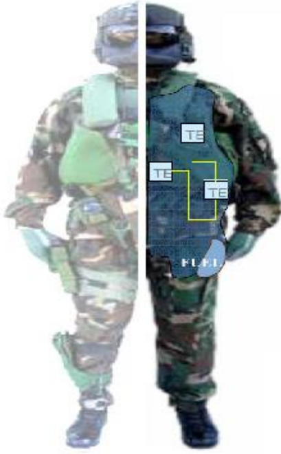
Fig. 3 Supplying the electrical energy requirement of a soldier with TEGs, therefore reducing the weight he carries.
