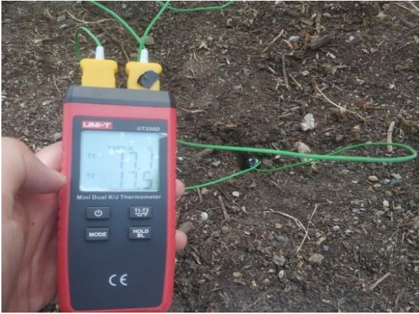
Fig. 6 This image of the thermometer was taken from 50 cm soil depth on 29.05.2021.
