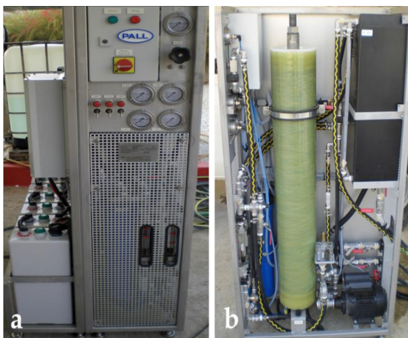
Fig. 1 First generation unit installed in rural areas. (a) external view; (b) internal view with the module, pump and cleaning tank.
