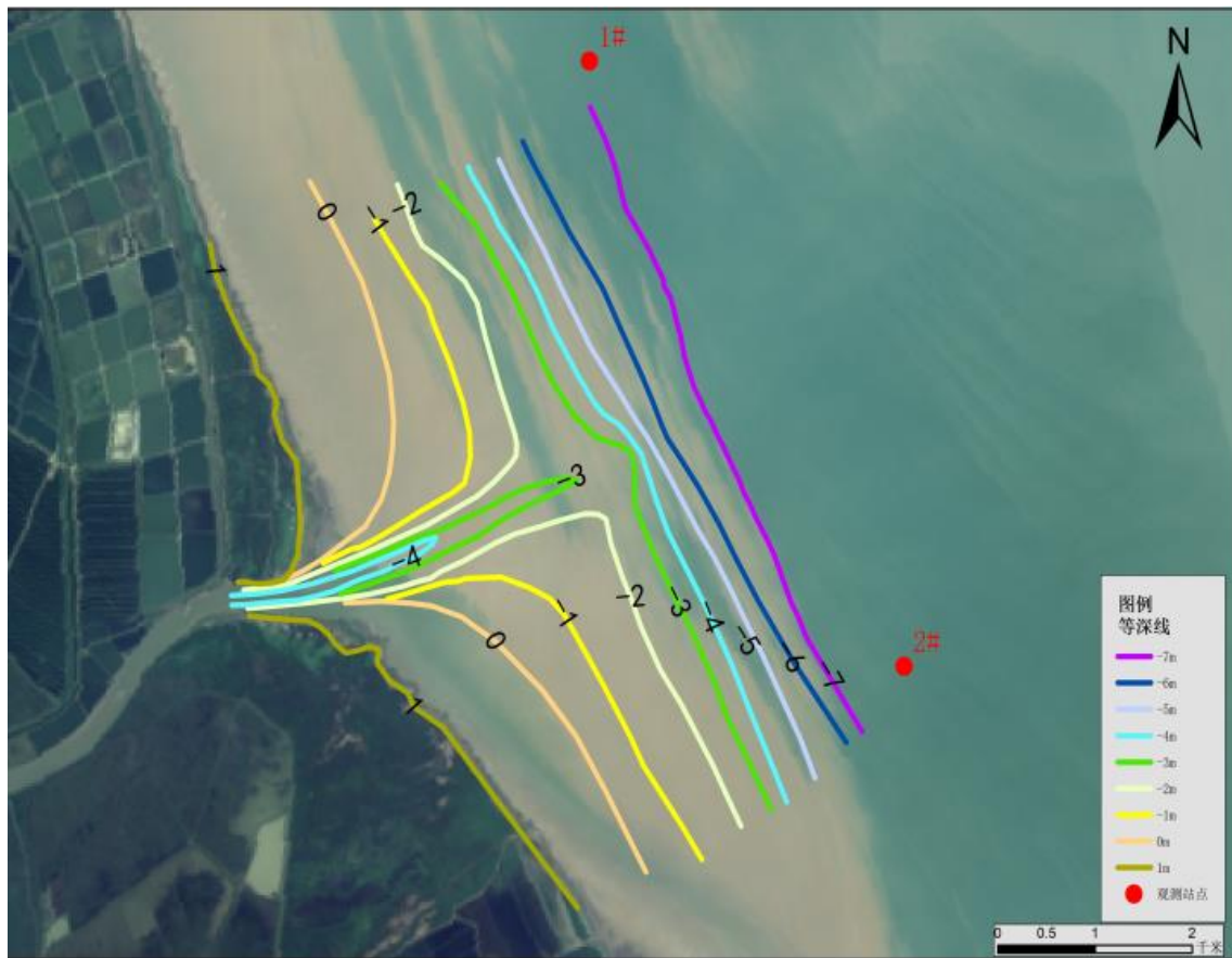
Fig. 9 Contour distribution of topography at the lower port road and outside the mouth of Xinyanggang Gate.
