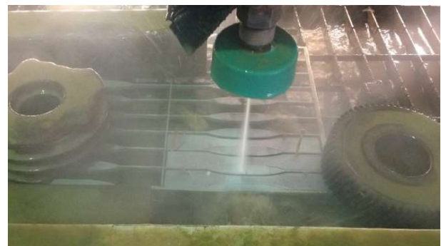
Fig. 1 Water jet peening process.
