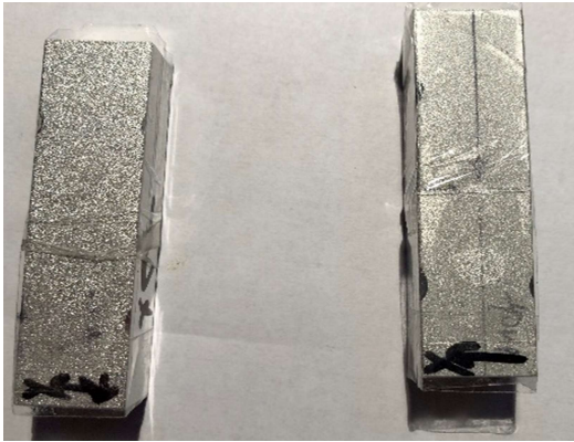
Fig. 2 Sample surface after shot peening.
