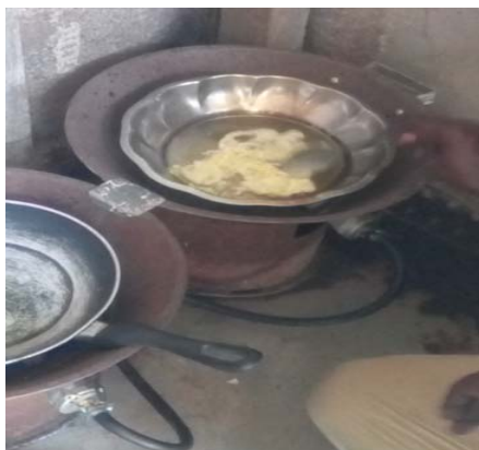
Fig. 4 Biogas combustibility test.
