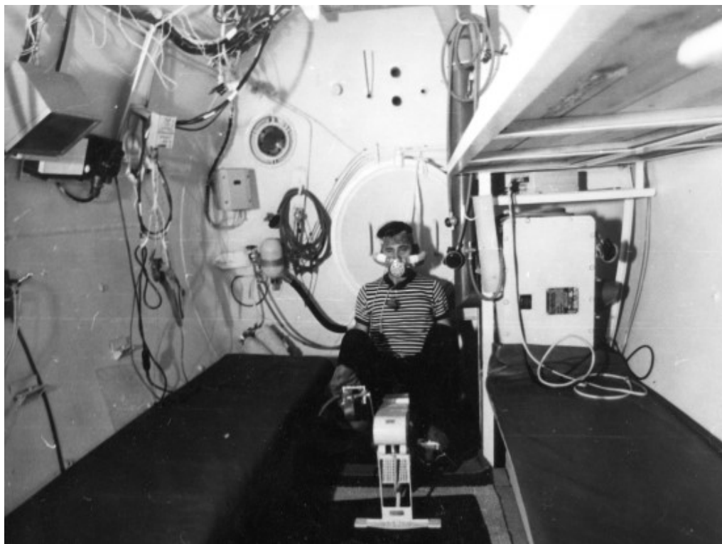
Fig. 3 Complex of hyperbaric chambers for saturation experiments ( N_2 + He/Ne + O_2 ) at “depths” of 450 m (Shirshov Institute of Oceanology of Russian Academy of Sciences, Gelendzhik, 1988).
