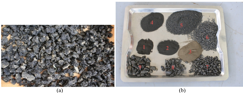
Fig. 5 RAP material: hand crushed (a) and gradation after binder extraction (b) [1 – 75 \mu m, 2 – 150 \mu m, 3 – pan, 4 – 300 \mu m, 5 – 600 \mu m, 6 – 5mm, 7 – 12mm, 8 – 14mm, 9 – 19mm].
