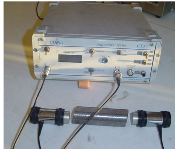
Fig. 5 Ultrasound tester CT-3 prepared for tests.
