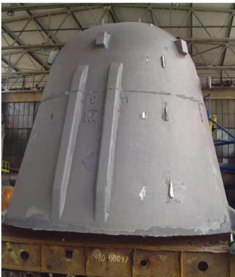
Fig. 8 Slag ladle of volume V = 15 \text{ m}^3 , produced of cast iron of a mixed graphite form, including vermicular.
