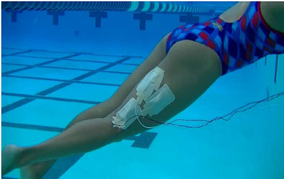
Figure 2. EMG breaststroke kick bicep (downward kick and horizontally kick).
