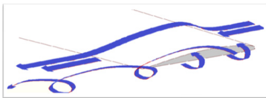
Fig. 4 Schematic drawing of the wing end vortex.
