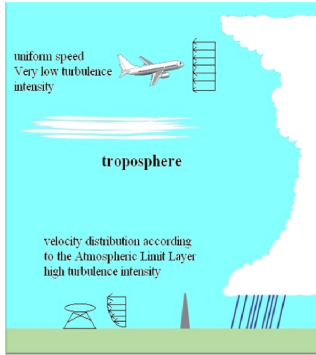
Fig. 5 Schematic drawing of velocity distribution.
