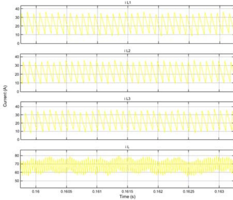
Fig. 3 DC/DC converter each phase and total current ripple.
