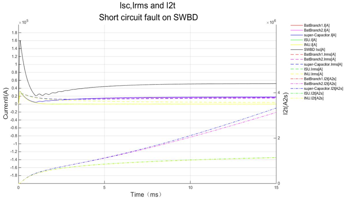
Fig. 5 Short-circuit currents, root mean square and  $I^2t$  for each branch.
