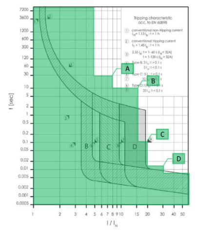
Fig. 3 BALIN tripping feature.
