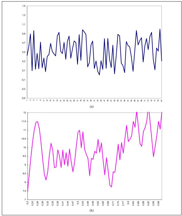
*Figure 9.* (a) stochastic process, generated by a random number generator; (b) Weierstrass function, where  $\varepsilon = 0.1$ ,  $\lambda = 1.1$ . Source: own research.
