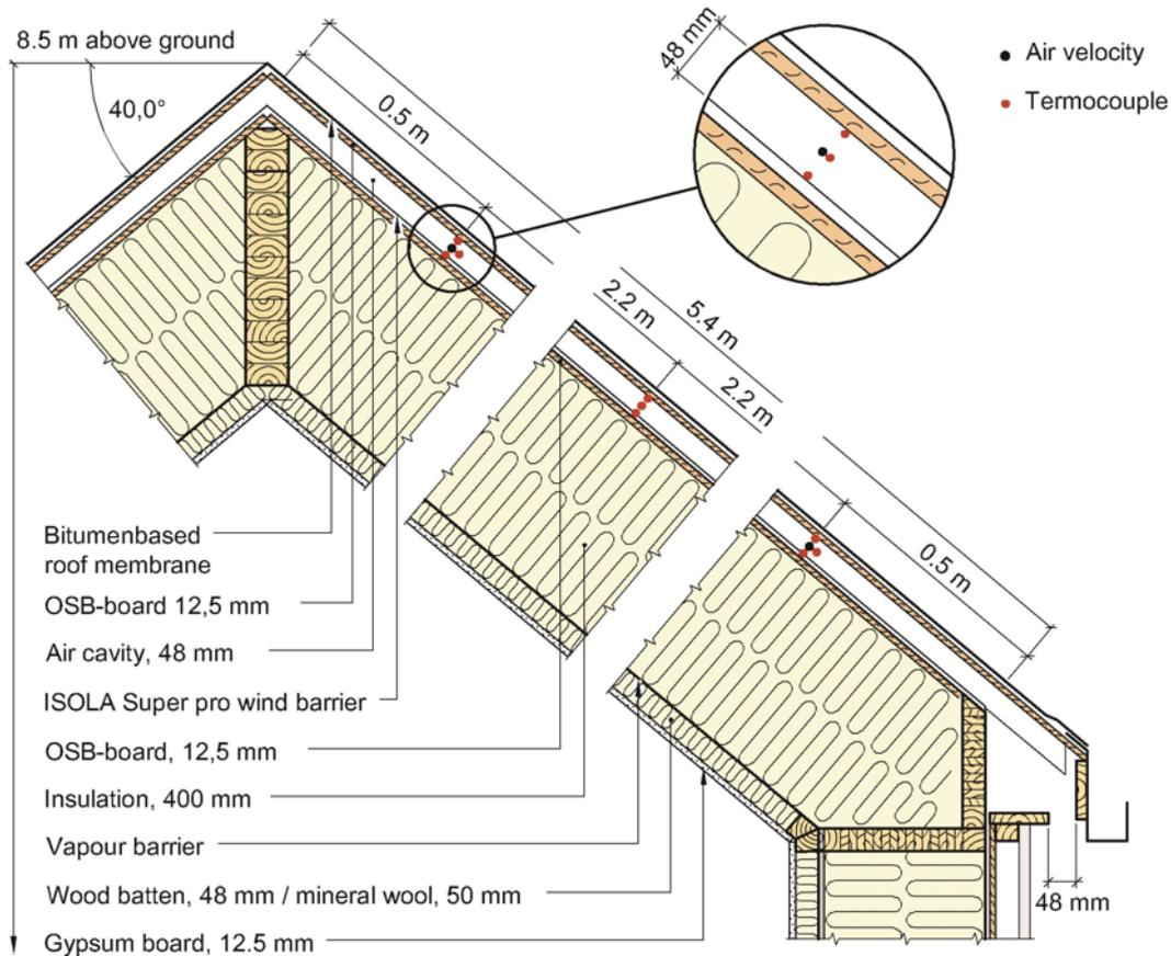
**Fig. 2** ZEB Test Cell Laboratory roof structure.
