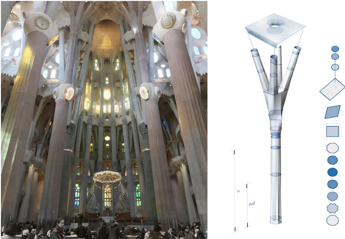
Fig. 11 (Left) the central atrium of the church; (right) pillar construction scheme. Source: the authors adapted of Ref. [21].
