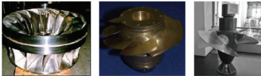
Fig. 6 Francis, Kaplan and propeller turbines.
