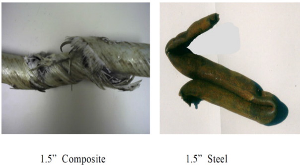
Fig. 5 Buckling Failure of Conventional Coiled Tubing under Compressive Force [36].
