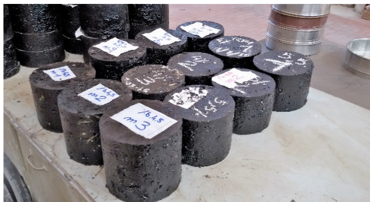
Fig. 20 Compacted SGC specimens of HMA_RFI 15 × 12 cm.
