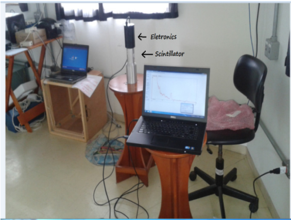
Fig. 1 View of the gamma scintillator with associated electronics and computer.
