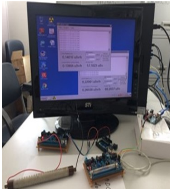
Fig. 1 Tubes (Russian and Chinese) with Arduino electronics and data acquisition with PC.
