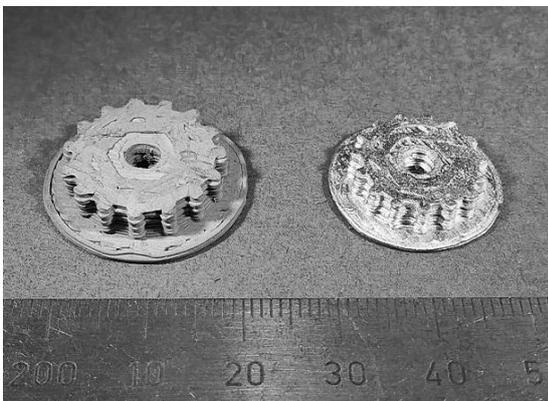
Fig. 3 Green part (left) and sintered part (right) of a pulley.
