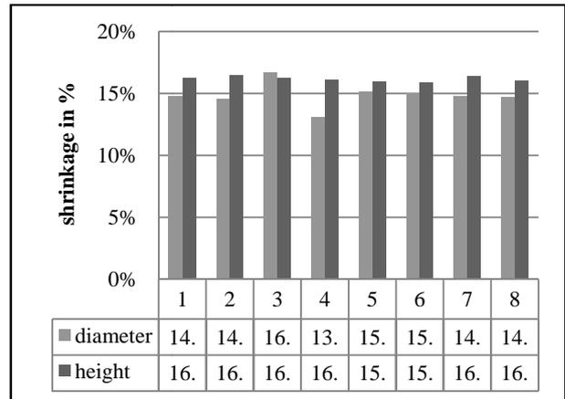
Fig. 4 Geometrical shrinkage of cylinders due to sintering.
