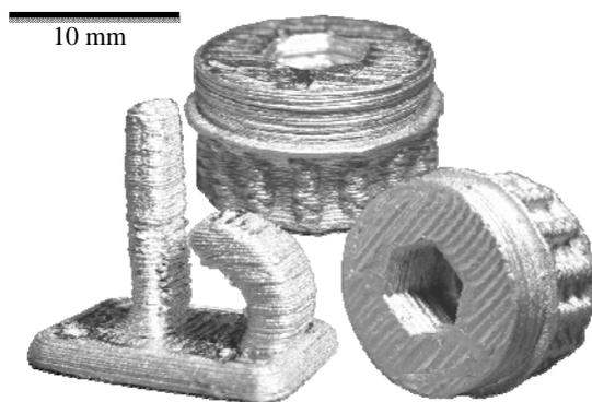
**Fig. 6** Different sintered components.
