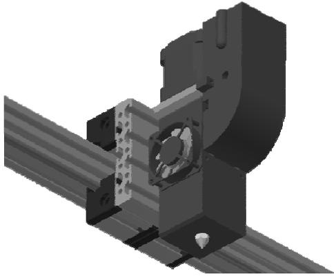
**Fig. 2** Moveable CEM extruder on x axis (CAD image).
