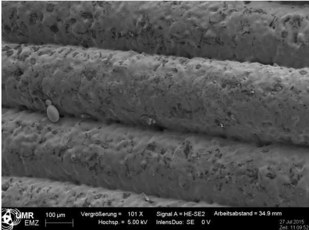
**Fig. 5** SEM image of a printed and sintered cylinder.
