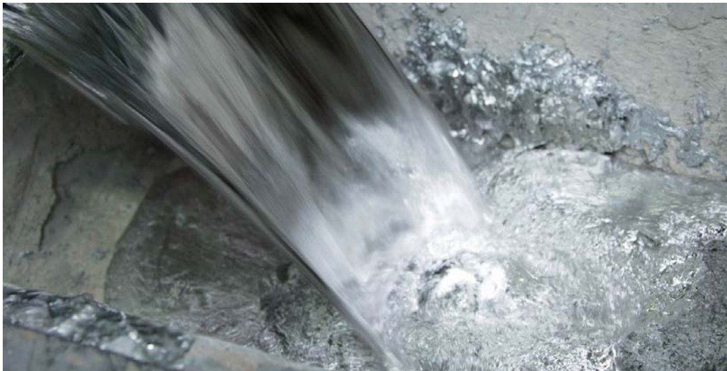
Fig. 3 Any interruption of the protective oxide skins on molten aluminium results in newly built, extremely thin oxide films.
