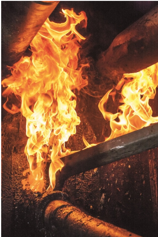
Fig. 6 Example for careless filling of the slot sleeve.
