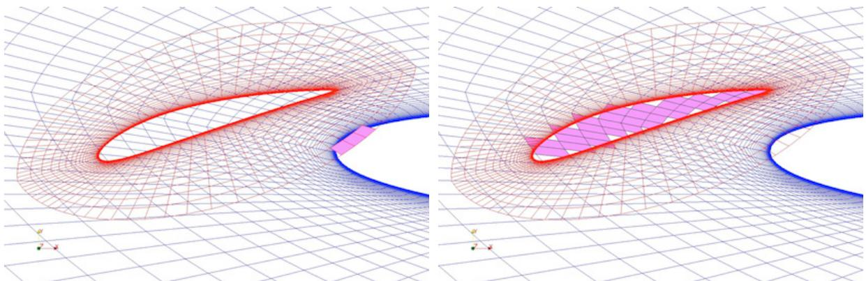
Fig. 4 left: in-wall cells of the slat grid, right: in-wall cells of the wing grid.
