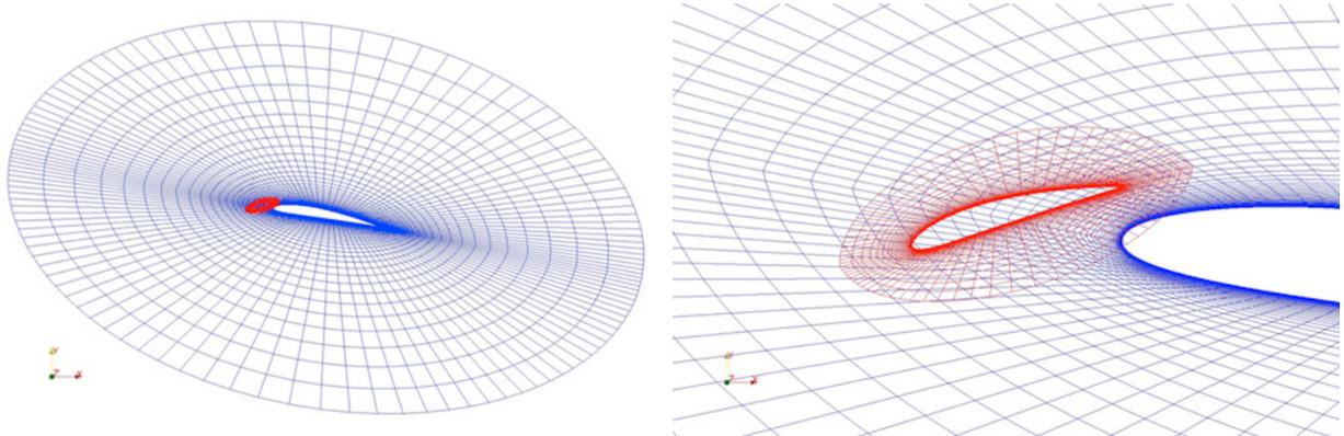
Fig. 3 Grid (Over view) and Zoomed to around the leading edge.
