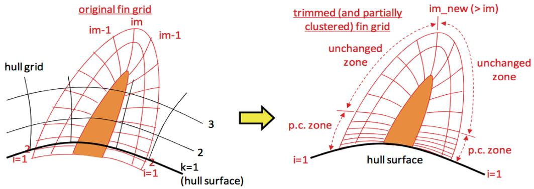
Fig. 1 Trimming and partial clustering (a fin attached to a hull): left: original, right: applied.
