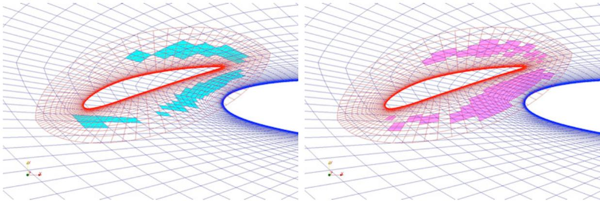
**Fig. 8** left: receptor o of the wing grid right: donor o of the slat grid.
