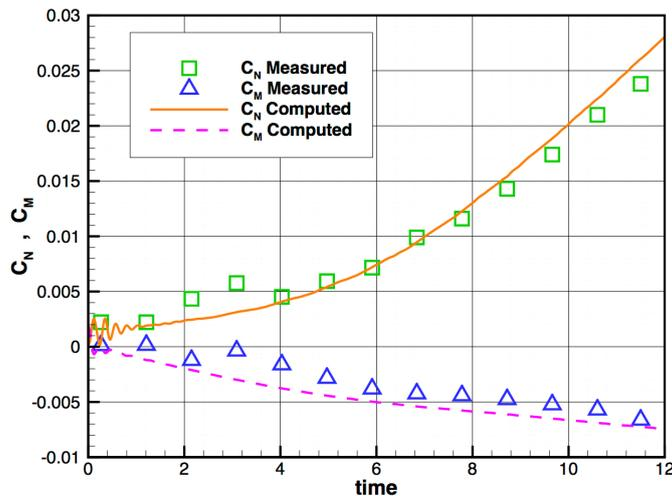
Fig. 13 Normal force ( $C_N$ ) and pitch moment ( $C_M$ ).
