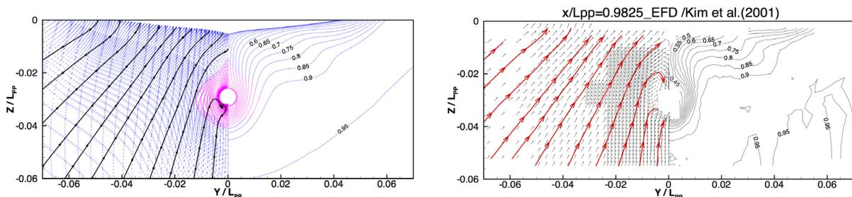
Fig. 11 Cross flow vectors and streamlines, (left) and axial velocity contours ( $\Delta U = 0.05$ ), (right) at  $x/L_{PP} = 0.9825$ . Top: Computed results, Bottom: Measured data
