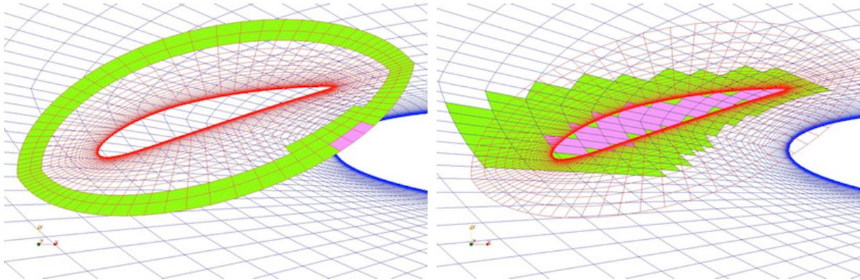
Fig. 5 left: receptor\_m cells of the slat grid, right: receptor\_m cells of the wing grid.
