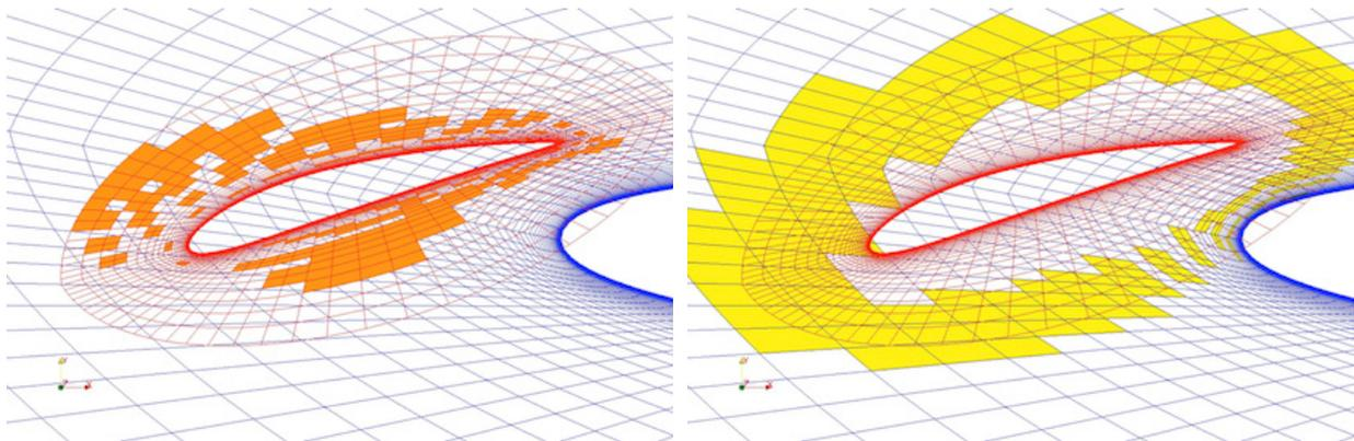
Fig. 7 left: donor\_m cells of the slat grid, right: donor\_m cells of the wing grid.
