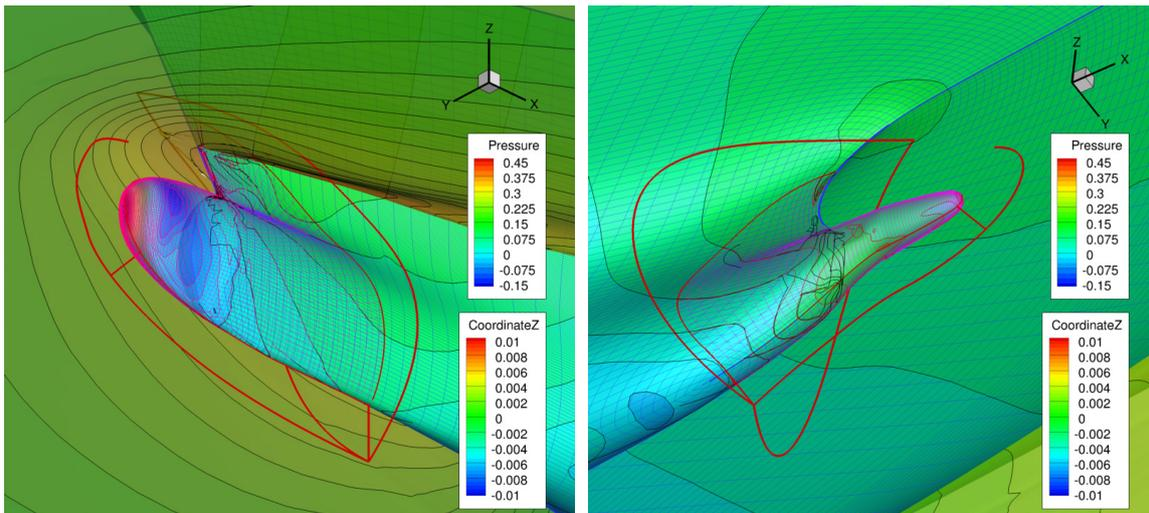
Fig. 10 Schematic view of bow (left) and stern (right). Pressure distribution on the hull surfaces and wave elevation ( $\Delta z/L_{PP} = 0.0005$ ) are also shown.
