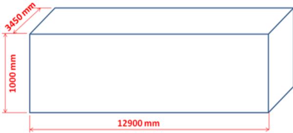
Fig. 5 Dimensions of stamped coal cake.
