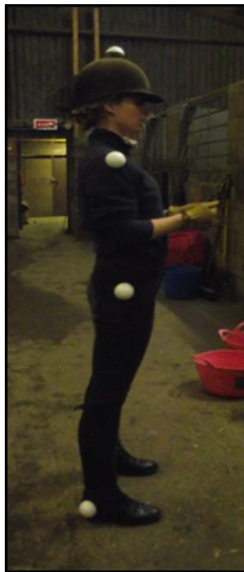
Fig. A2 Marker placement on rider indicating anatomical landmarks to determine ESHH.
