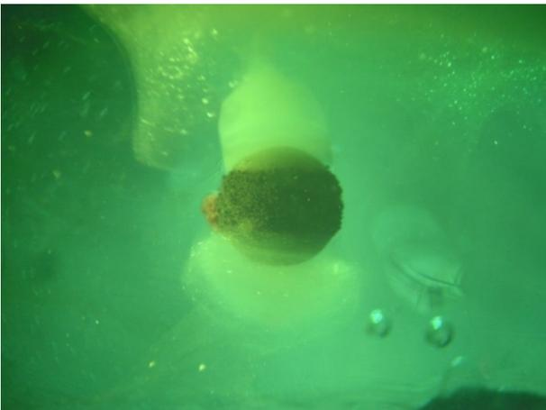
**Fig. 6** The process of deformation of the regions with high concentration of  $\text{Fe}^{2+}$  clusters. The ball diameter  $d = 4$  mm.
