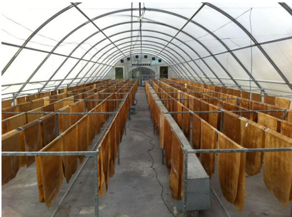
Fig. 3 The natural rubber sheets dried inside the dryer.
