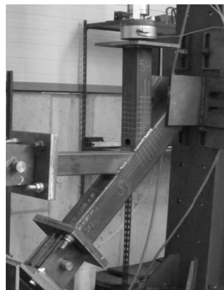
Fig. 1 Test configuration for K-joints.
