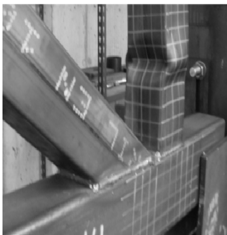
Fig. 6 Failure in a N-joint without the vent hole.
