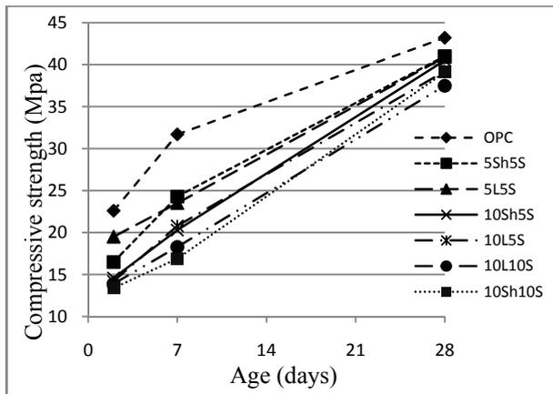
**Fig. 4** Strength development of cement samples.**Table 5** Properties of concrete samples.
