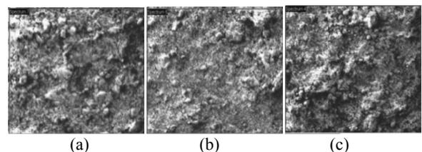
**Fig. 3** Microstructure of: (a) OPC; (b) 5L5S; (c) 5Sh5S.
