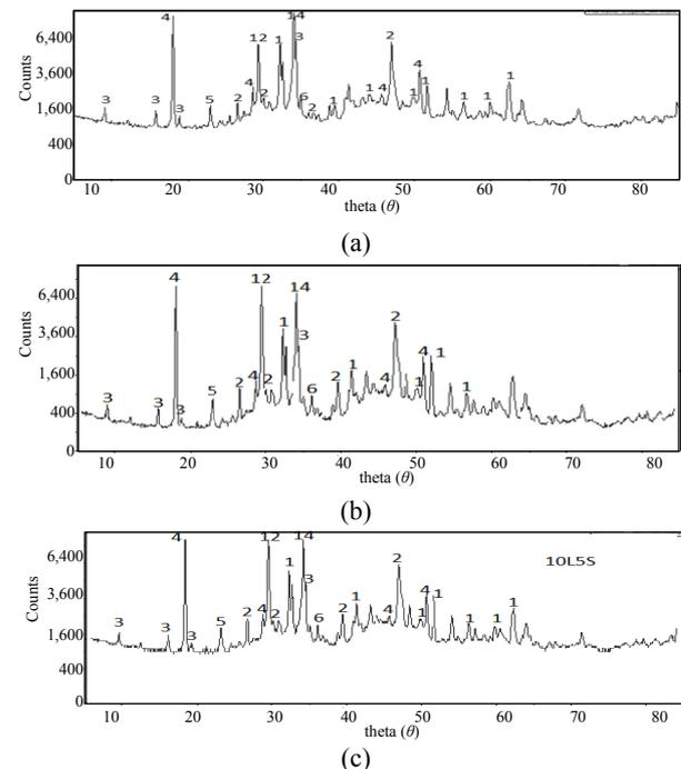
**Fig. 2** X-ray diffraction graphs of OPC and blended cements at 28 days (1—C<sub>3</sub>S; 2—C<sub>2</sub>S; 3—ettringite; 4—Ca(OH)<sub>2</sub>; 5—C<sub>3</sub>A; 6—Quartz).
