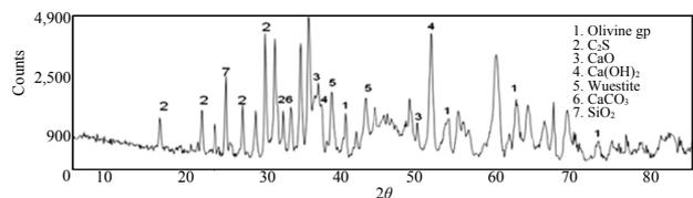
**Fig. 1** X-ray diffraction graph of steel slag.
