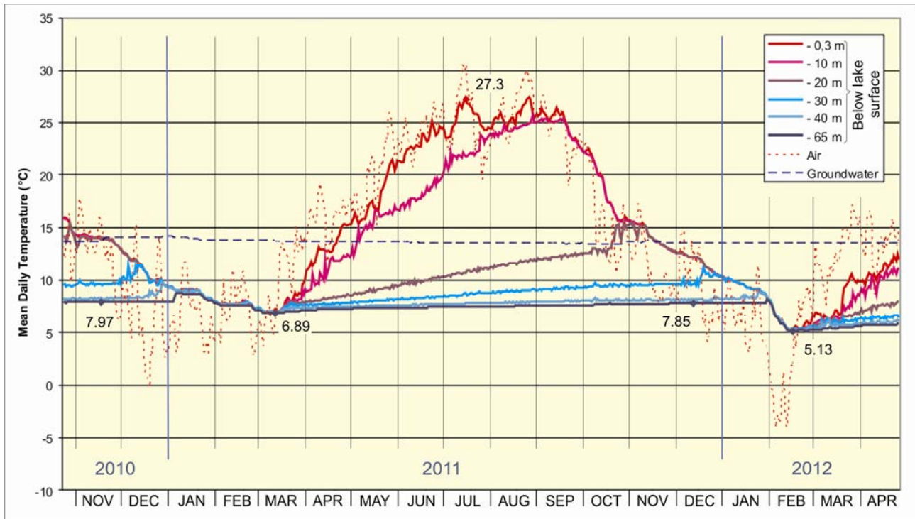
Fig. 4 Mean daily water temperature fluctuations on different depths of the lake in comparison with temperatures of air and groundwater.
