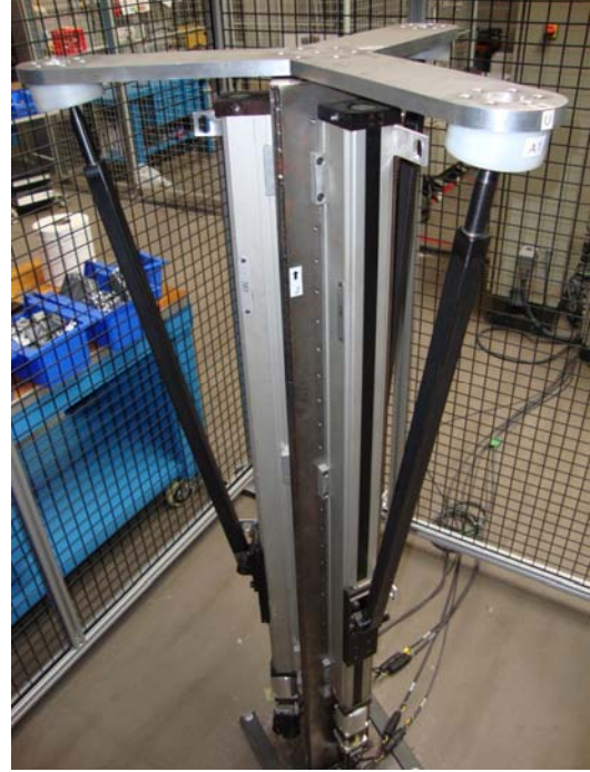
Fig. 3 3- \underline{P}RS parallel manipulator prototype.
