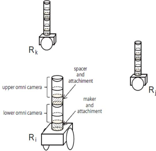
Fig. 1 Outline of the distance measurement using two omnidirectional cameras.
