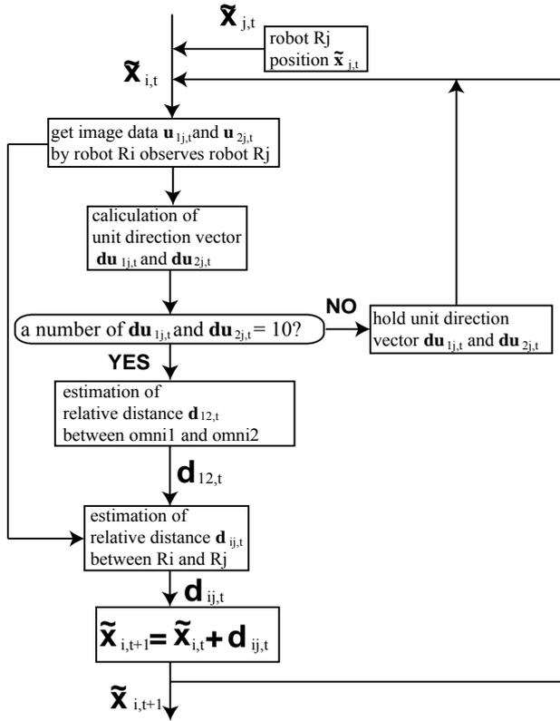
Fig. 3 The flow chart of the self-position estimation of the mobile robot.
