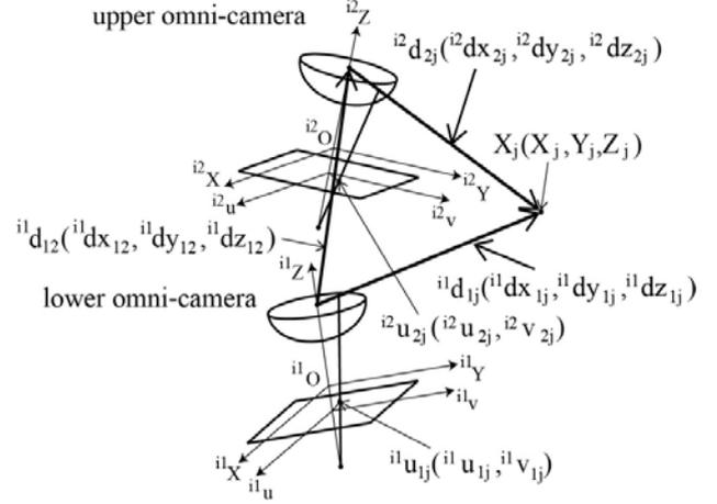
Fig. 2 The geometric relation of two omnidirectional cameras equipped on the robot Ri and the marker equipped robot Rj.
