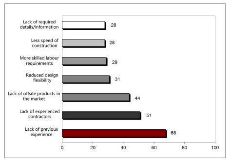
Fig. 6 Main barriers for using offsite methods (%).
